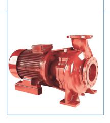
The Armstrong 4030 Starnorm and 4280 Starbloc Series offer technical excellence with a compact configuration. Both designs feature DIN 24960 mechanical seals with carbon vs. silicon carbide faces for long life and a pull out design for easy maintenance.
