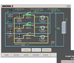
The IPP-CHW solution is available as a variable primary flow configuration or a variable primary/variable secondary configuration. Units can be configured to include an optional variable flow roof mounted cooling tower, or a cooling tower can be connected on-site separately.
