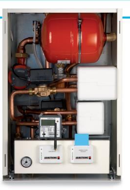
A wall mounted unit with one plate heat exchanger that separates the apartment's domestic hot water circuit (DHW) from the central supply. The apartment's heating circuit is fed directly from the central supply.
