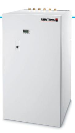
A floor standing unit with one plate heat exchanger that feeds the apartment's heating circuit or, via a 3-port valve, an integrated unvented DHW storage cylinder.
