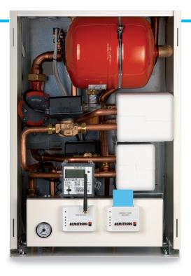
A wall mounted unit with two plate heat exchangers; one separates the apartment's heating circuit and the other separates the apartment's domestic hot water circuit (DHW) from the central supply.
